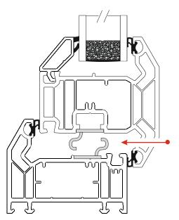
STAY GUARD ELITE SG036 on outer frame and sash for types of stay to include Egress/Easy Clean
